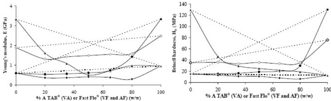
**Figure de gauche:** Young's modulus ( $E$ , interpolated values) as a function of binary mixture composition ( $\alpha = w/w_{tot}$ , %) for various compact mean compositions.
